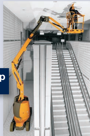
Gelenk-Teleskop - articulated telescopic boom
